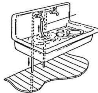
FIGURE 2: Pipe-to-Water Cross Connection. A cross connection is created when the hose is submerged in water in the sink.
